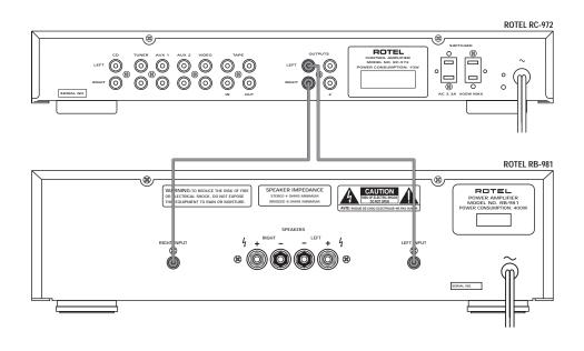
Figure 4: Line Level Input Connection
